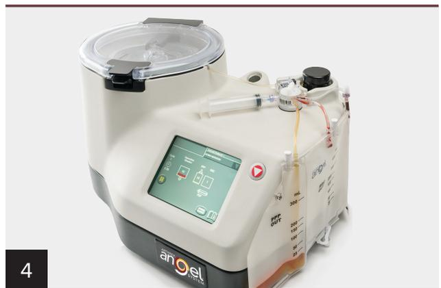
The first component to be collected is PPP. The Angel system will stop collecting PPP when the 470 nm wavelength of light is absorbed by platelets. The Angel system will turn the valve to collect PRP until RBCs are detected by the absorption of the 940 nm wavelength of light.
