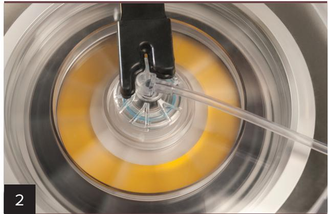
The Angel system can process 40 mL to 180 mL of whole blood in a single cycle. The first component to be harvested is the platelet-poor plasma (PPP) followed by the platelet-rich plasma (PRP). The red blood cells (RBCs) will be collected last in the RBCs Out compartment. The approximate spin time for 40 mL of whole blood is 15 minutes. The spin time for 180 mL of blood is 26 minutes.
