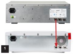
Connect the red cable that comes with the CW4 to the rear of the Synergy Resection Console
