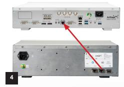
\*Connect to the Synergy imaging console for the heads up display
