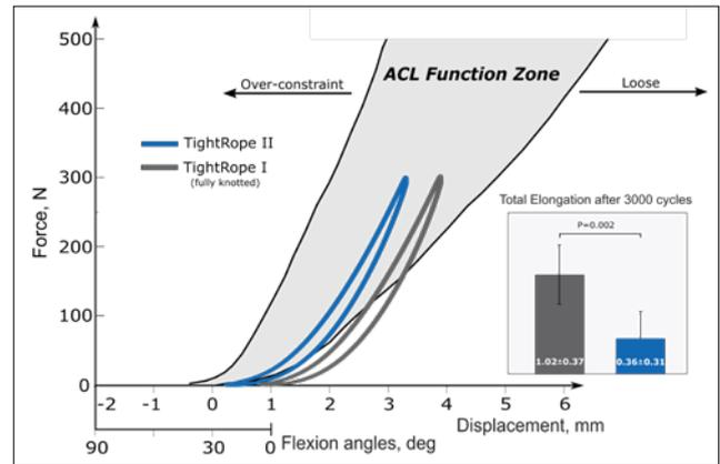
**Figure 4.** Final loading situation at the end of testing with significantly less elongation for TightRope II constructs in reference to the native ACL behavior<sup>1</sup>
