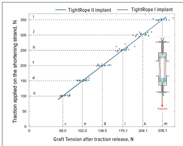
**Figure 3.** Linear regression analysis of the tensening data over all traction levels
