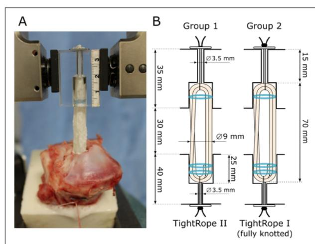
**Figure 1.** Experimental setup (A) with schematic illustration of bone tunnel and graft-related definitions (B)
