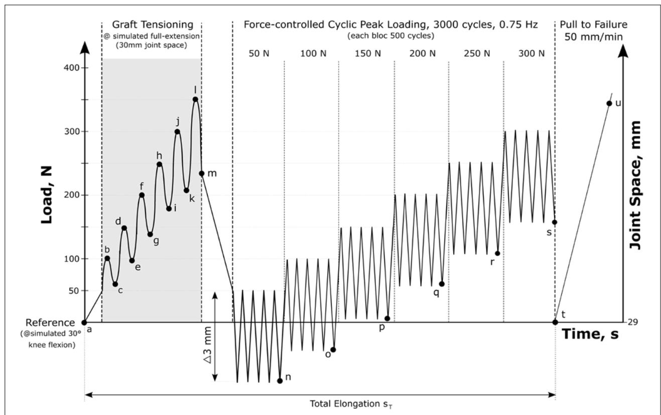
**Figure 2.** Test methodology with graft tensiing, cyclic and pull-to-failure loading protocol
