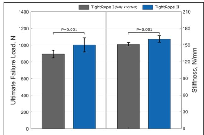
**Figure 5.** Ultimate failure load and stiffness test results
