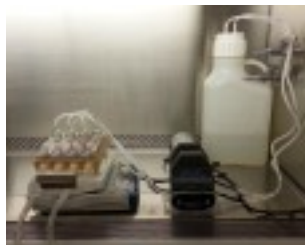
Fig. 2. Set up of a colony drip-flow reactor (DFR) biofilm applied with sample dressings (left) and preparation of antimicrobial efficacy testing in colony DFR biofilm model (right). Sample dressings were applied directly onto the biofilms that continuously deposited onto hydrophobic filter membranes for 72 h incubation at room temperature.
