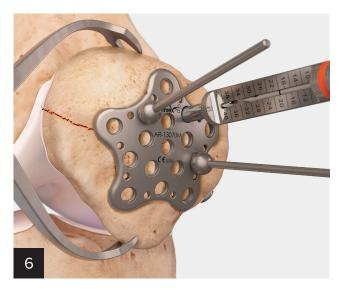
Screw a drill/depth guide into the locking holes before drilling. Screw length is determined by referencing the laser line on the 2.0 mm drill bit at the scale on the drill/ depth guide.
