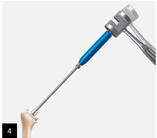
4 Once the appropriately sized implants have been determined, thread the stem / cup impactor handle securely to the CA adaptor. Then impact the implant onto the Univers Revers suture cup, taking care to ensure the tab of the CA adaptor is aligned with the lateral slot of the suture cup.
