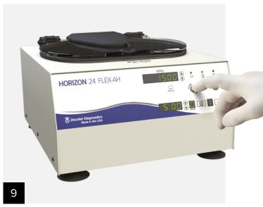
Run the centrifuge at 1500 rpm for 5 minutes.
