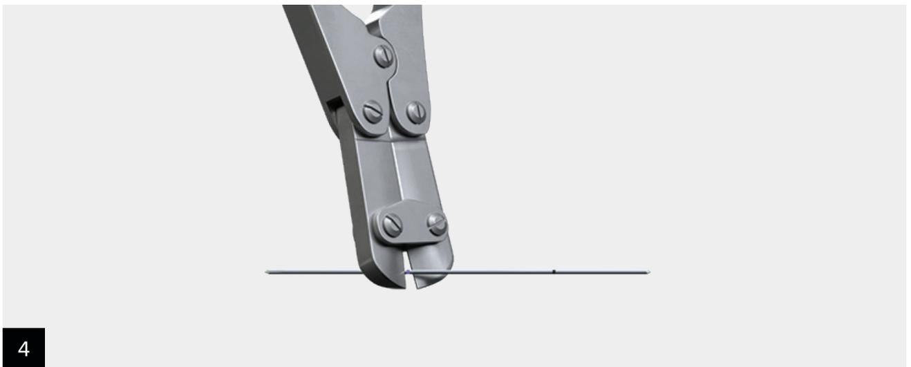
Cut the wire at the marked line. To aid in insertion, cut the FlexWire at an angle to create a bevel.
