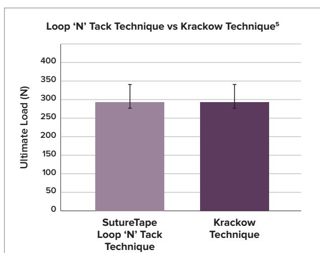
In biomechanical testing, the suture configuration used for the Loop 'N' Tack technique was shown to be equivalent in strength to the standard Krackow stitch with no significant differences in ultimate load and cyclic displacement. The stiffness of the suture configuration was significantly greater than that of the Krackow samples.<sup>5</sup>
